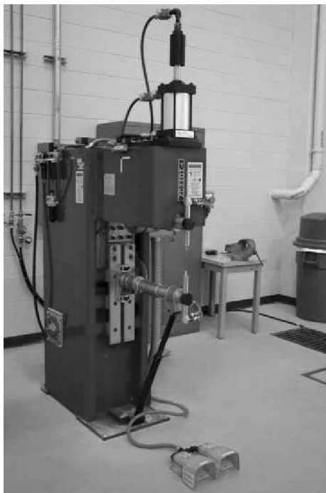
FIGURE 7.2 Pedestal-type spot welder.
