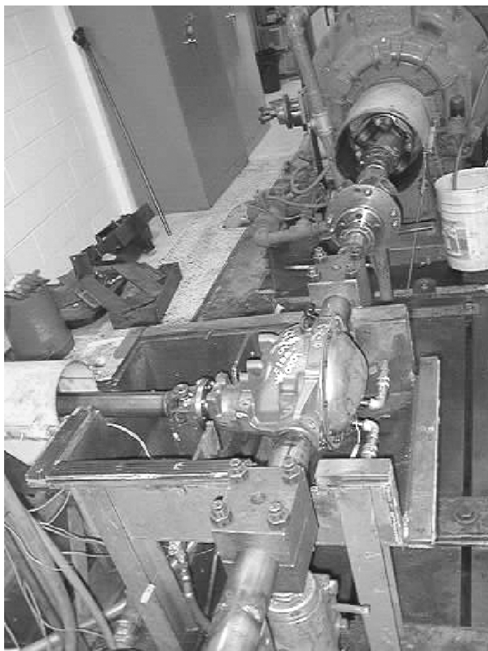
FIGURE 8.2 A rear differential dynamometer test setup.
